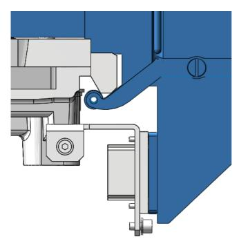
Step 4: release the handlebar and lock in the feeder bank
